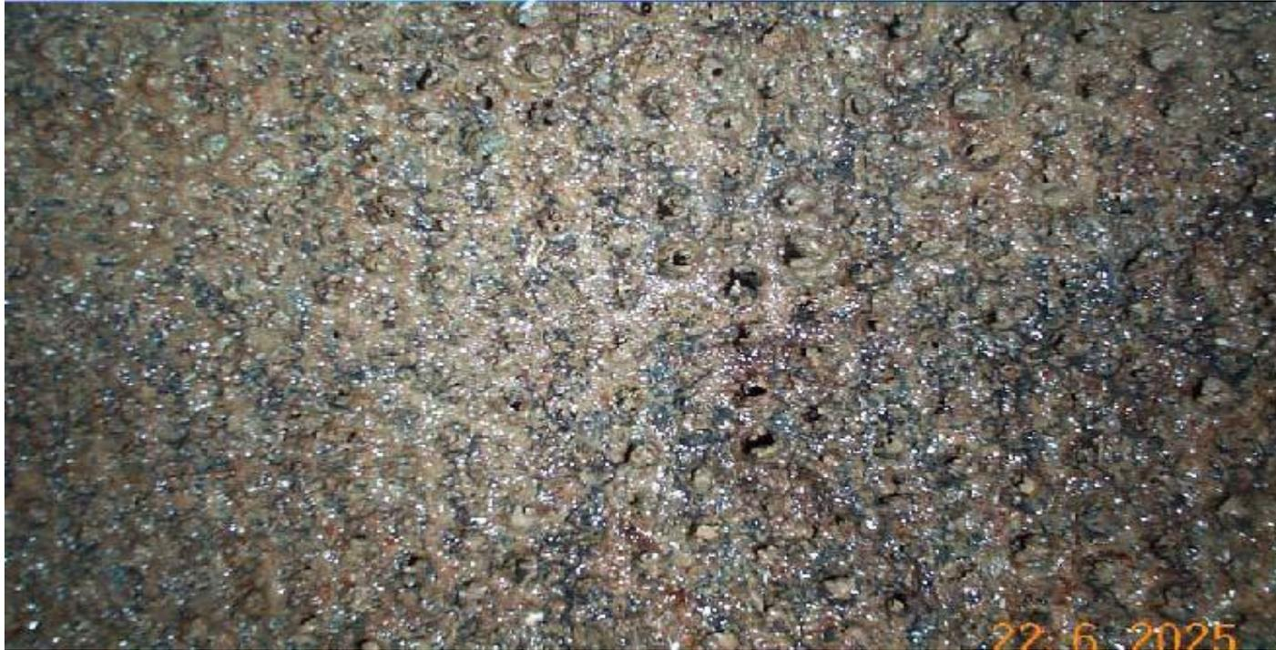
Heat exchanger treated with chlorine
